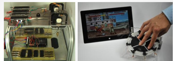
An artificial muscle computer (left) and an artificial muscle sensor for human computer interaction.
