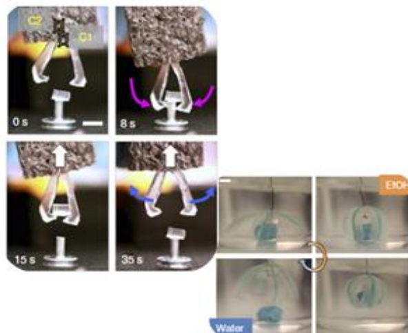
Figure 4 Soft tweezers (left) and soft gripper (right) made from hydrogels handling small parts of polydimethylsiloxane. Image from Palleau et al , Nature Comm., 2013.
