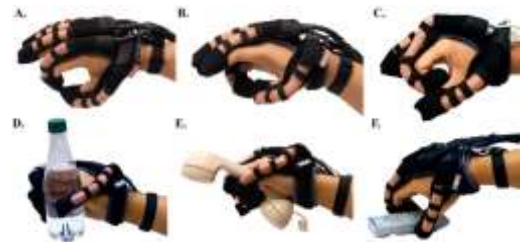
Figure 4: The soft robotic glove in: A. index finger - thumb opposition contact, B. small finger -thumb opposition contact, C. index finger flexion, D. grasping a bottle of water using all fingers, E. picking up a telephone using all fingers, except of the small, and F. grasping of a television remote control using a tripod pinch. Figure reproduced from [4].
